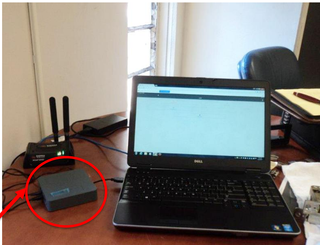
Cellular station, gateway and user device (PC)
