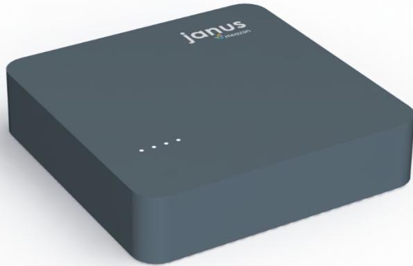
A Linux-based, small form factor appliance for provisioning, aggregating and backhauling data from Meazon's metering and sensor devices to online Meazon's Cloud Gateway service over Ethernet. Thanks to the user-friendly provisioning web application UI, minimal configuration effort is required even for large scale deployments.
